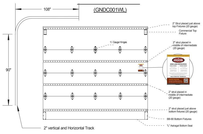
~Note: The use of 2" track with clip style continous jamb brackets are required and fastened to jamb with 3/8" x 3" lag screws.
